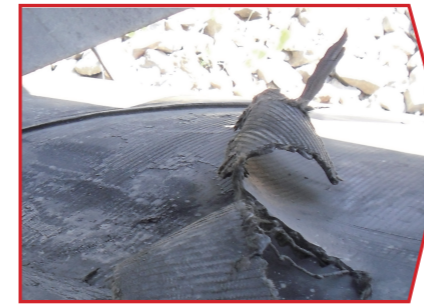
The vulcanized area has torn from the splice and ripped into the SBR belt.
