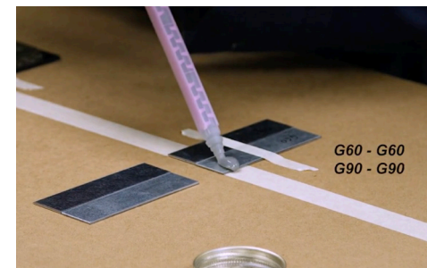
Plexus MA 8100 testing shows bonding of composites, metals and dissimilar substrates
