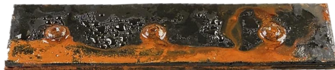
Corrosion and moisture intrusion in environmentally aged samples
